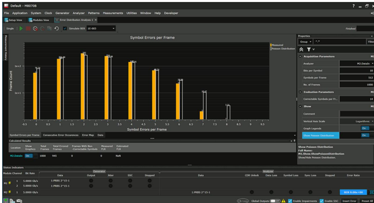
Figure 25. The error distribution analysis M8070EDAB provides multiple views to debug the error distribution. The figure shows an example of symbol errors per frame based on captured pattern streams, with the measured frame loss ratio, based on user-definable number of bits per symbol, correctable symbols per frame and frame length.
